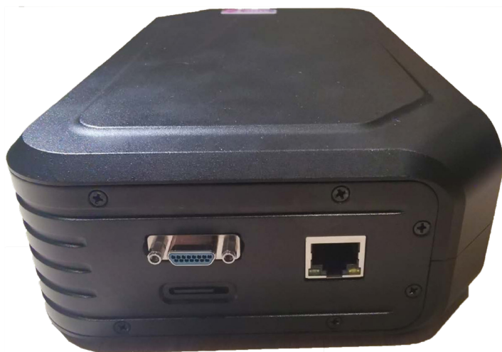
Corona Camera Basic Unit (Mounted into the rugged housing)
